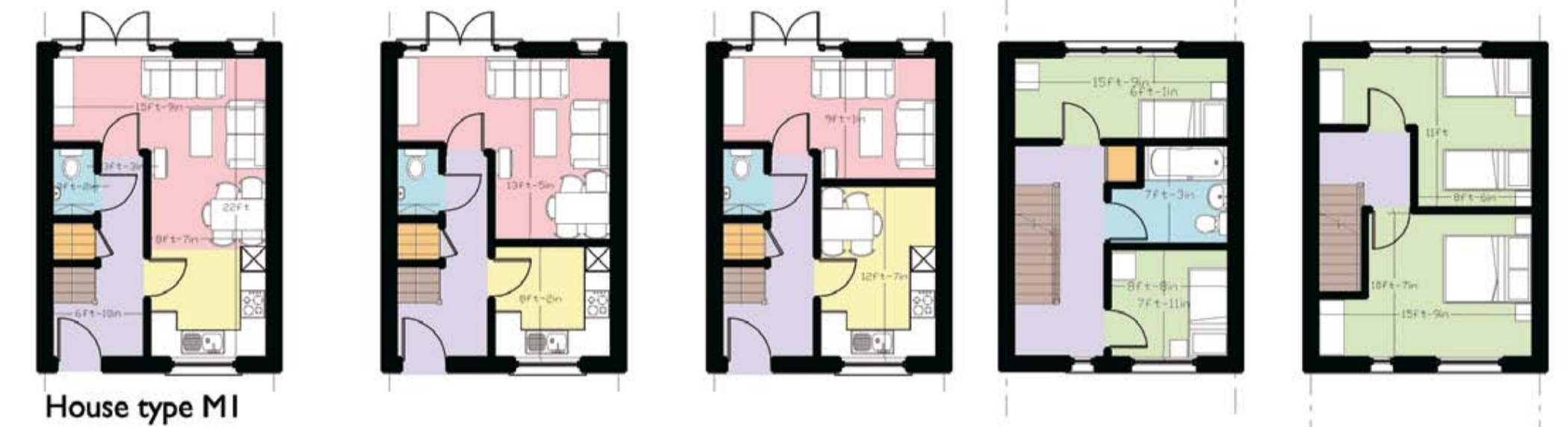
Ground Floor Option 1 Ground Floor Option 2 Ground Floor Option 3 First Floor Second Floor
